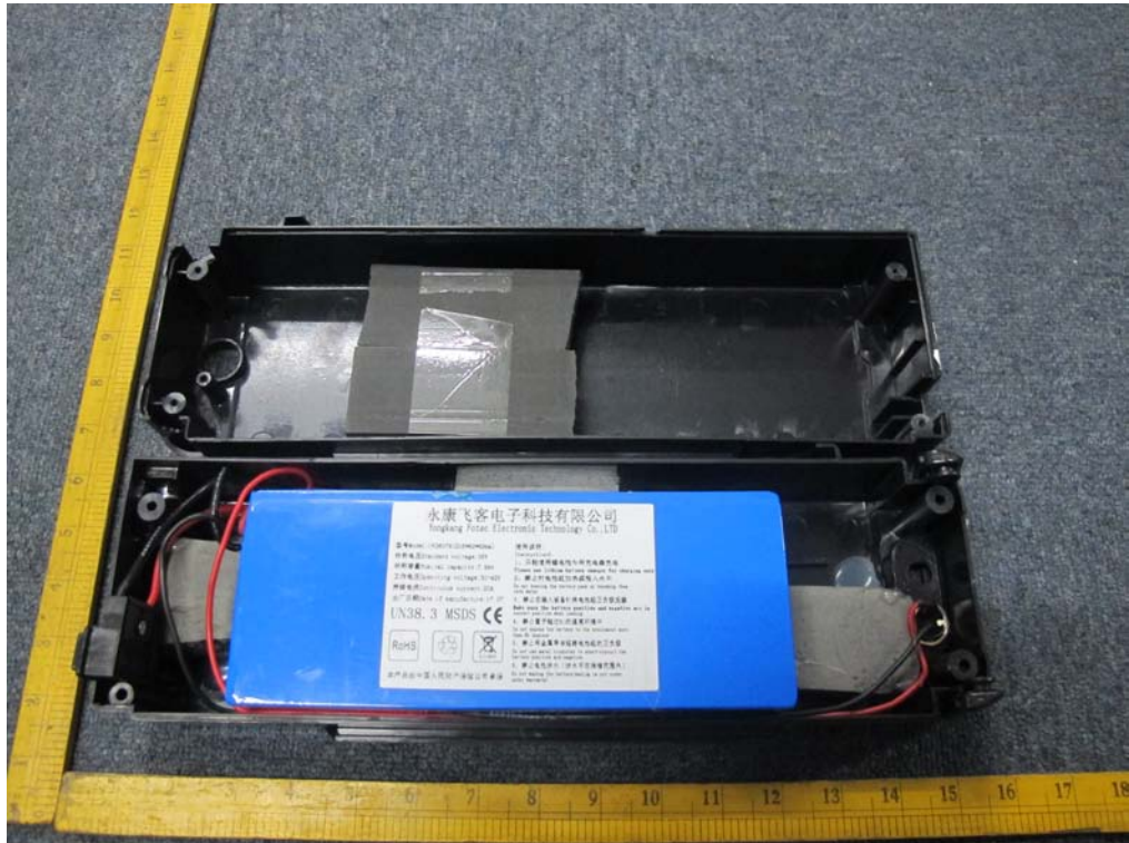
Figure 3 Internal view of Battery
